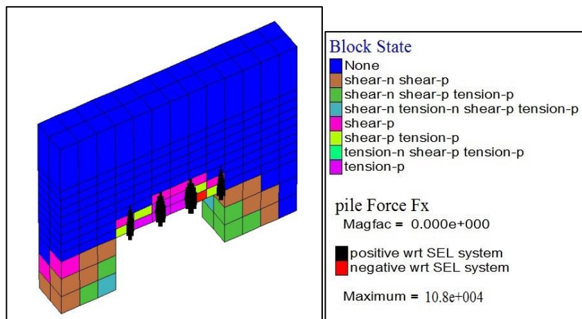
Figure 6.11 Maximum value of axial load on bolt and roof yield at instrumented rock bolt location GSG1 for GDK-5A, Incline, SCCL
