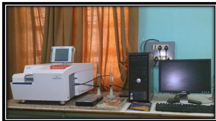
Figure 2.5: Photograph of TGA used in material analysis (Mettler-Toledo).
