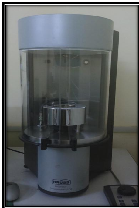
Figure 2.7: Photograph of Tensiometer used in identified wettability of different material analysis (Krüss F-100 tensiometer).
