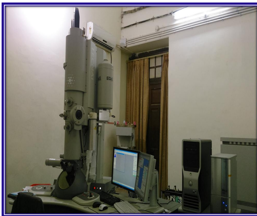
Figure 2.9: Photograph of TEM used in identification of morphology of different polymer composites.
