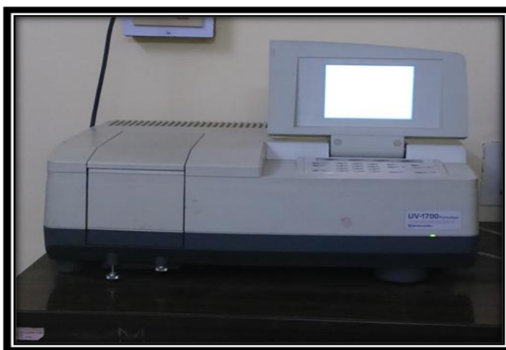
Figure 2.2: Photograph of UV-Visble used in material analysis (Shimadzu (UV-1700), Pharma Speck).
