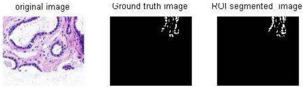
Figure 3.3(b): Original, Ground truth and ROI Segmented by FCM segmentation
