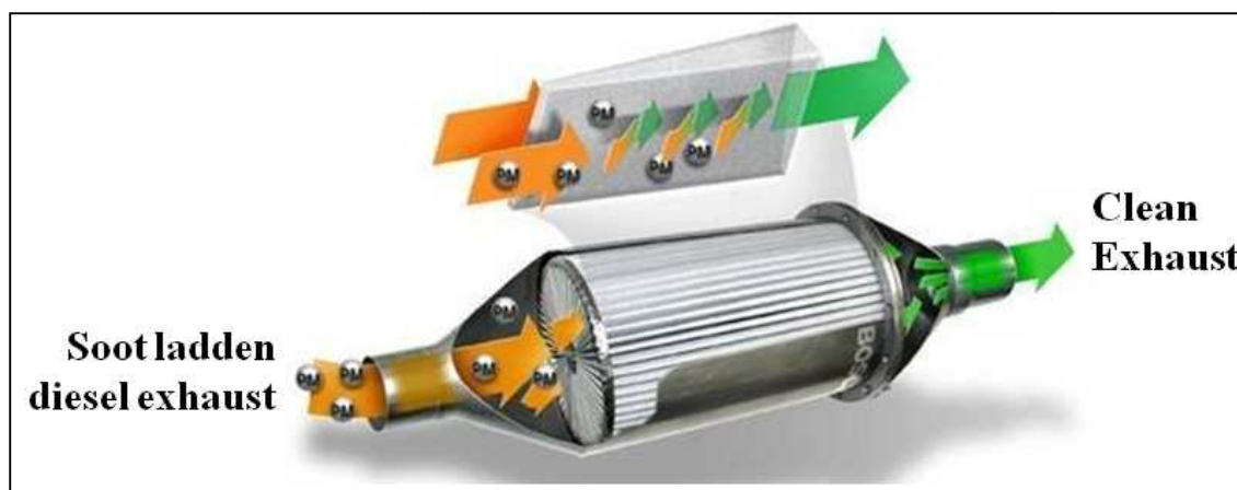
Figure 1.12 Schematic diagram of DPF
