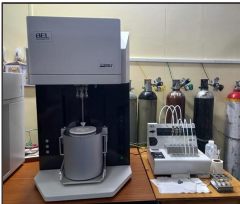
Fig. 2.9 Photograph of the Surface area measurement instrument. (Courtesy: CIF, IIT (BHU))
