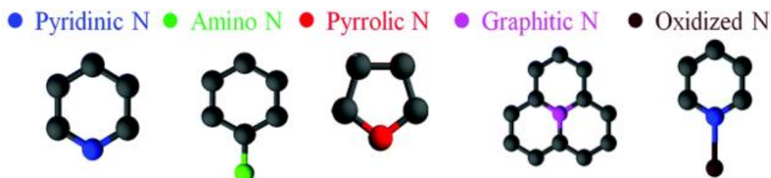
Fig. 1.11 Different bonding states of nitrogen atoms into the carbon (graphene) atmosphere. Reprinted with permission from Ref. [46] (License ID 1173032-1) Copyright@2021 The Royal Society of Chemistry.
