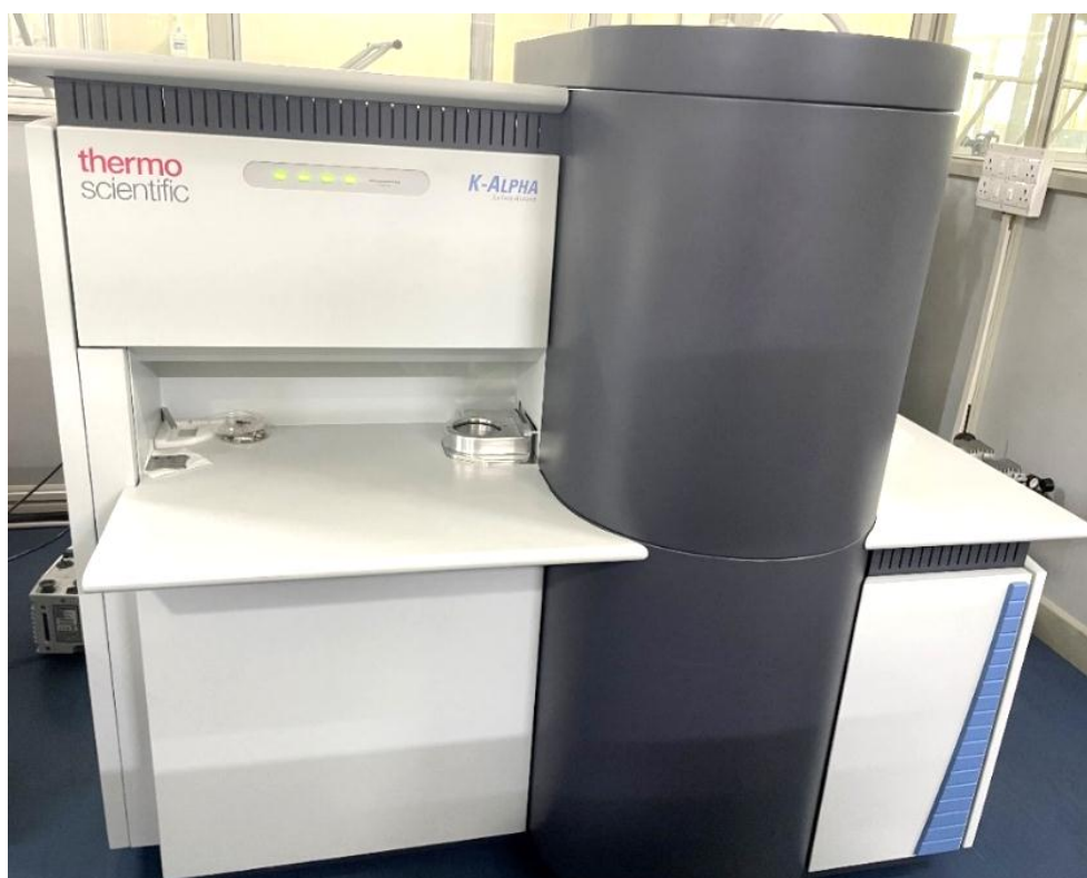
Figure 2.13: Shows the instrument for analysing X-ray photoelectron spectroscopy (XPS) (K-alpha, XPS dispersive spectrometer, Thermo Scientific).
