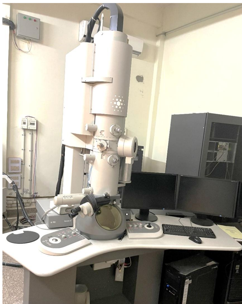
Figure 2.12: Shows a transmission electron microscope (TECNAI G2 20 TWIN, FEI-USA) equipped with the energy-dispersive X-ray spectroscopy (EDX) used for analyzing nanostructures for this research work.
