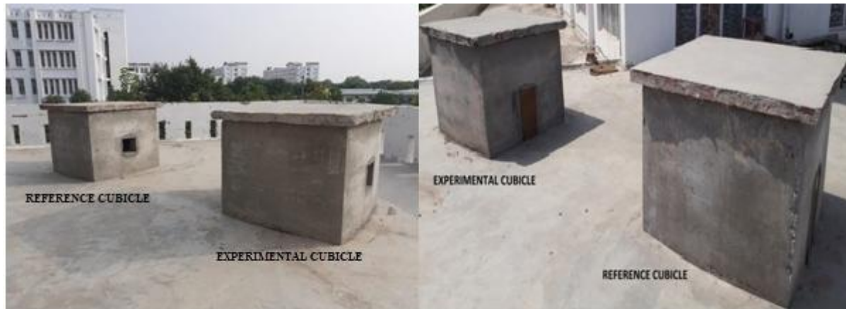
Figure 3.7 Experimental setup photographs of developed experimental and reference cubicle
