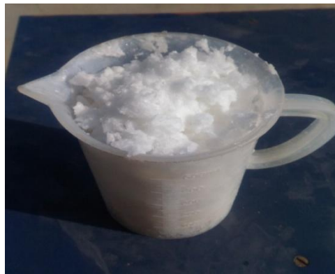
Figure 3.1 Commercially available OM37 PCM
