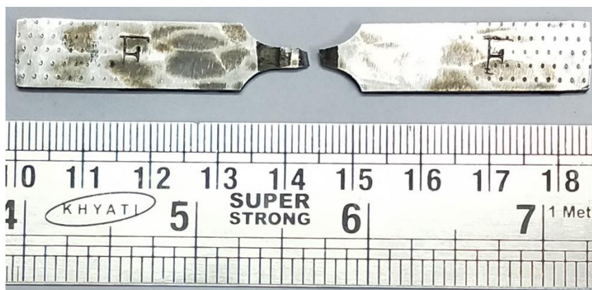
Figure 3.32 Fractured reduced section tensile sample after performing tensile testing.
