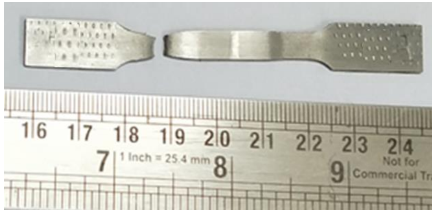
Figure 3.31 Fractured transverse tensile sample after performing tensile testing.
