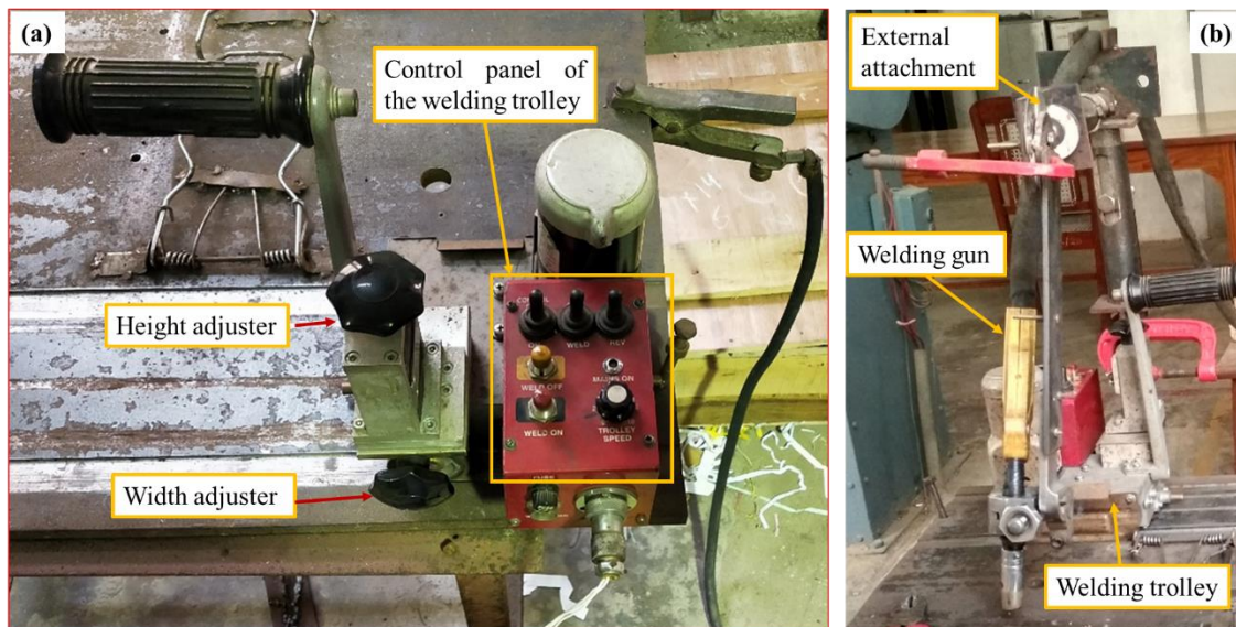
Figure 3.5 Welding trolley: (a) controller components, (b) attachments to the welding trolley.
