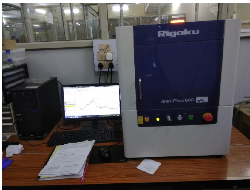
Figure 2.6: Experimental setup of X-ray diffractometer CIF IIT (BHU) [Rigaku Miniflex II, Japan]
