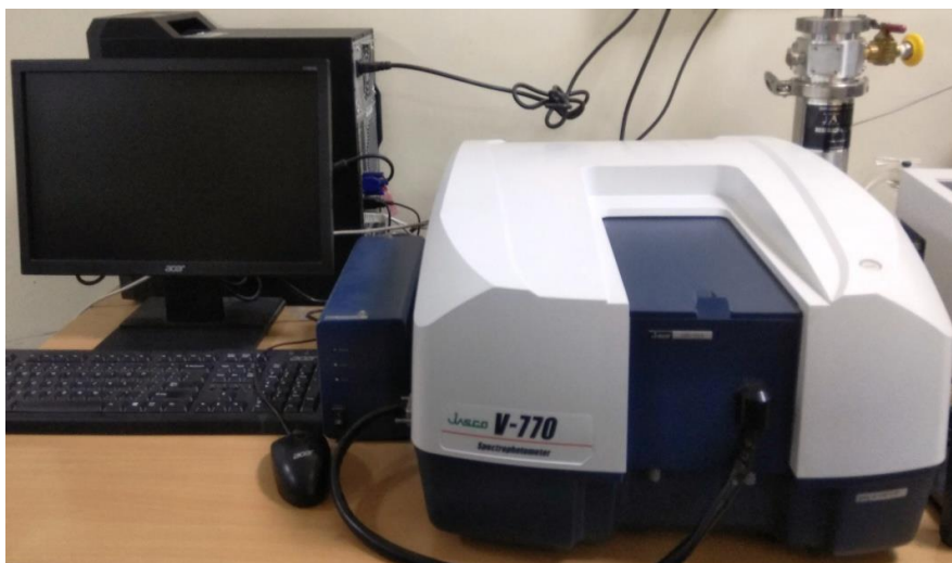
Figure 2.14: Experimental setup of UV-Visible measurement[JASCO V-770 UV-Vis spectrometer]
