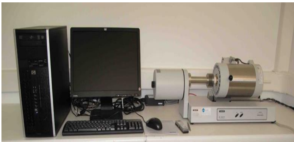
Figure 2.8: Experimental setup of Dilatometry for TEC measurement [NETZSCH DIL, 402 PC/4]
