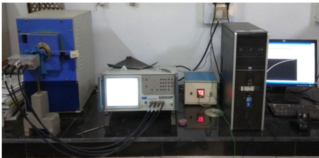
Figure 2.17: Experimental set up of automated impedance analyzer along with sample holder and furnace (6500 P Wayne Kerr, UK)
