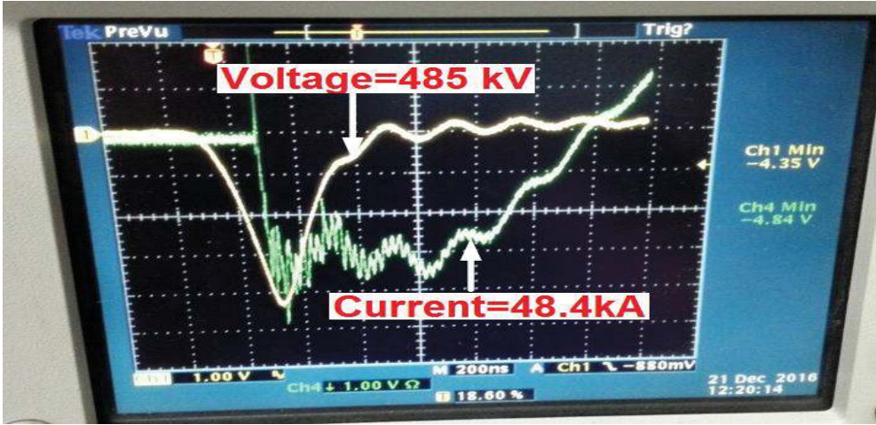
Fig. 6.15 : Measured voltage and current Waveform of MILO
