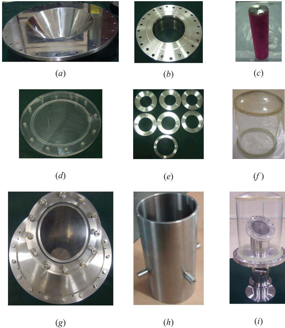
Fig. 6.13: Fabricated piece parts of MILO (a) Conical Flange (b) Vanes support (c) Cathode pasted with velvet (d) Window (e) Vanes (f) Bell jar (g) Vlasov antenna (h) Beam dump (i) Final assembly of MILO.
