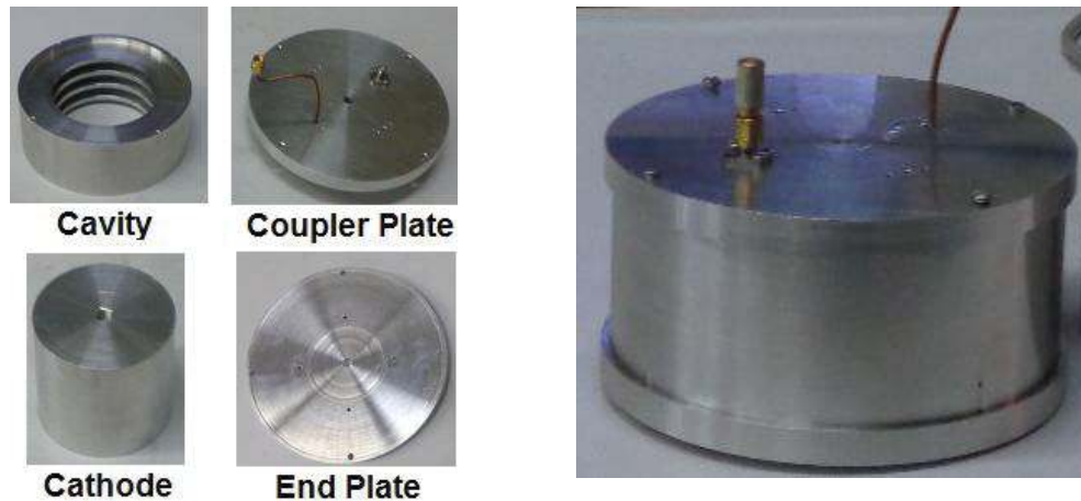
Fig. 5.3: (a) Fabricated piece parts of RF Interaction Structure and (b) Assembly of interaction structure
