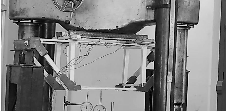
Figure 2.2 Buckling test experimental setup
