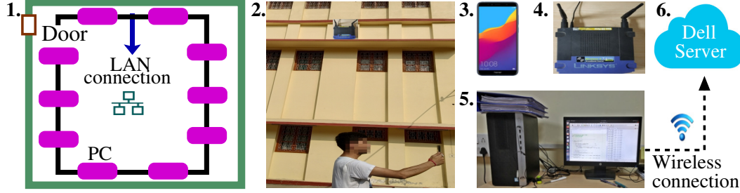
Figure 5.4: Prototype components: (1) PCs organization in the lab, (2) prototype deployment area, (3) smartphone, (4) router, (5) PC in lab, and (6) DELL server as Cloud.
