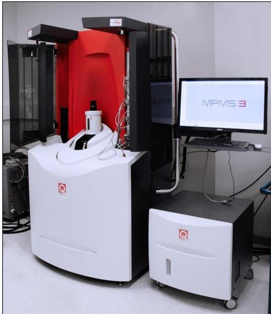
**Figure 2.9:** MPMS-3, Quantum Design (USA) used for magnetic measurement
