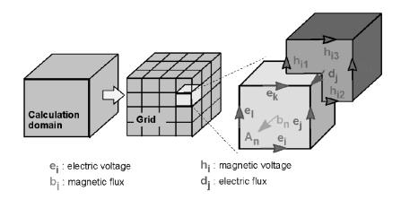
After completion of griding of a calculation domain, Maxwell's equations are formulated for each cell facets separately and done the calculation accordingly.
