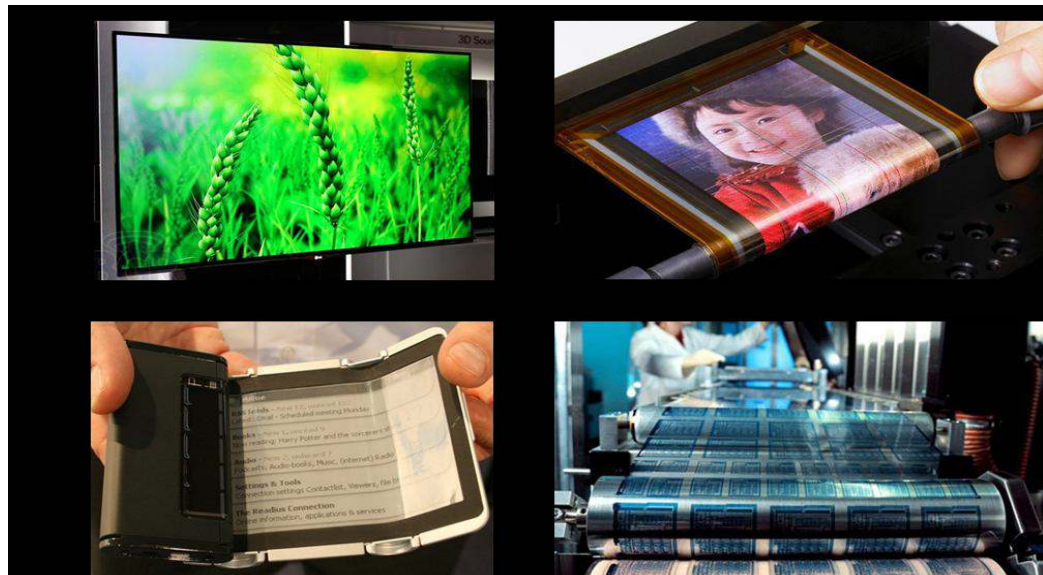
Fig. 1.17 (a) LG Electronics: the world's largest OLED HDTV presented at the 2012 Consumer Electronics Show (CES) in Las Vegas, it has a display size of 55 inches, weighs a mere 7.5 kg and is only 4 mm thick [Electronics (2012)], (b) Sony: a rollable full color 4.1 inches OLED display driven by OFETs, being wrapped around a thin cylinder [Sony (2010)], (c) Polymer Vision: 'Radius', a flexible electrophoretic (e-ink) display fabricated on plastic substrates using OFET backplanes [Polymer vision (2008)], (d) Poly IC GmbH & Co. KG: roll-to-roll printing organic RFID tags on plastic substrates [Poly IC (2012)].
