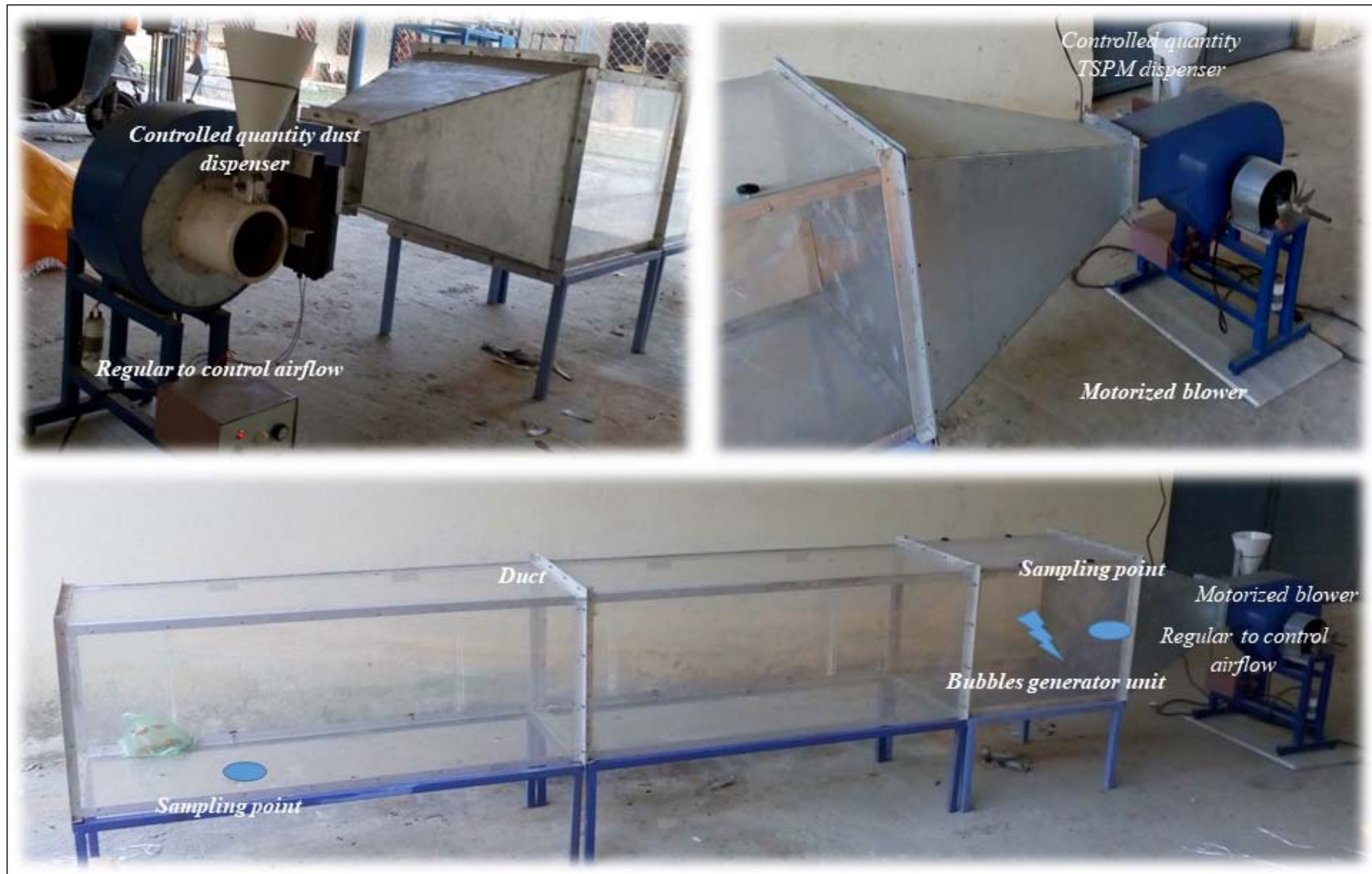
Fig. 10.3: Dust scrubbing set up to study the effect of bubbles on TSPM suppression
