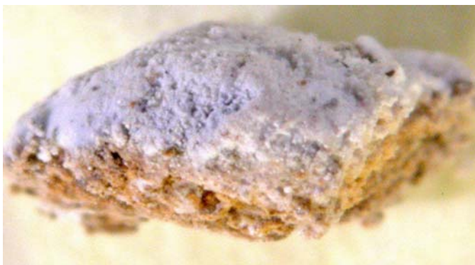
Fig. 4 (online colour at: www.pss-a.com ) Cross section of the reaction product obtained from Si-NP kept at 1350 °C during 15 minutes. Sample mass 5.29 mg.
