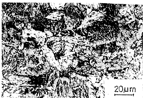
Fig. 10. Microstructure photograph of stationary prepared weldment (grain size = 38 μm).
