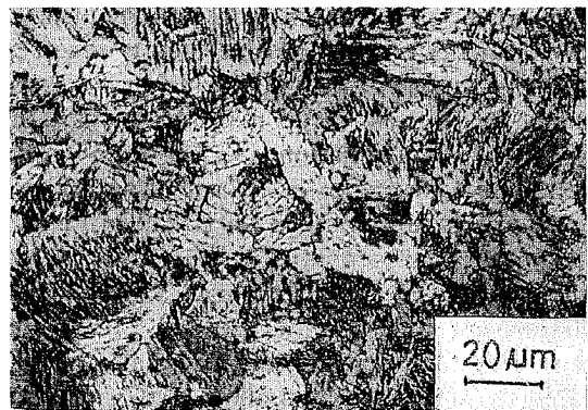
Fig. 8. Micrograph of stationary prepared weldment (grain size - 38 \mu\text{m} ).
