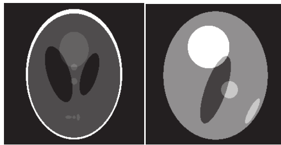
Fig 5.1: The phantoms used in the simulation study, Modified Shepp-Logan phantom (128 x 128 pixels), CT Test phantom (128 x 128 pixels)
