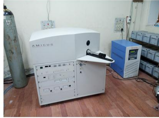
Figure 2.8: Mechanism (left) and experimental setup (Amicus) of X-ray photoelectron spectroscopy
