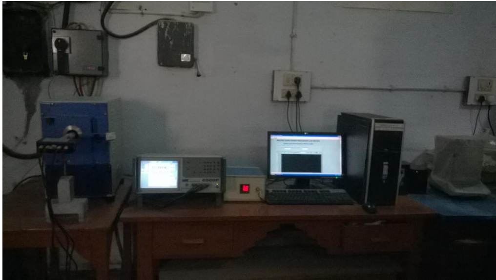
Figure 2.11: Computer controlled automated impedance analyzer setup along with sample holder and furnace (6500 P Wayne Kerr, UK)
