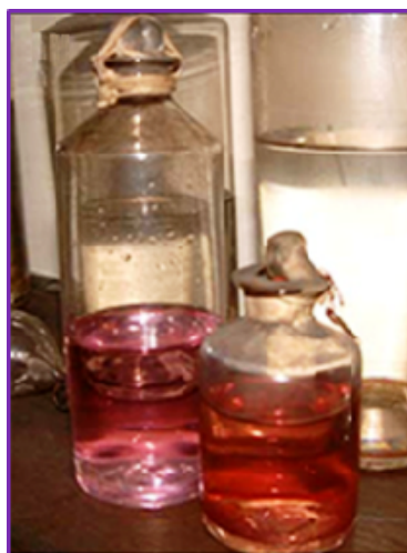
Figure 1.4: Faraday is credited as the discoverer of metallic colloid, he prepared gold colloids that were purple red in color by the reduction of gold salts with phosphorous, courtesy– Royal Institution of Great Britain available from: http://www.rigb.org/rimain/heritage/faradaypage.jsp .
