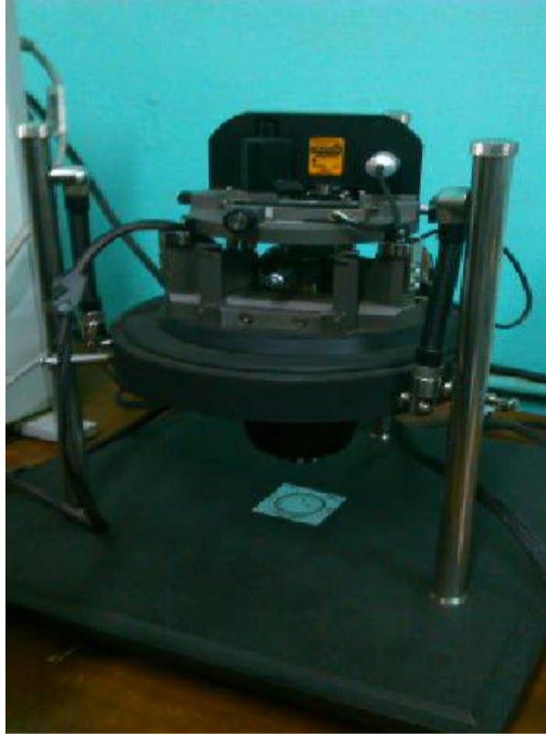
Figure 2.7 Atomic Force Microscope, model Pro 47, NT-MDT, Russia
