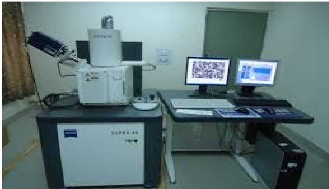
Figure 2.6 Scanning Electron Microscope, SUPRA 40, Carl Zeiss, Germany
