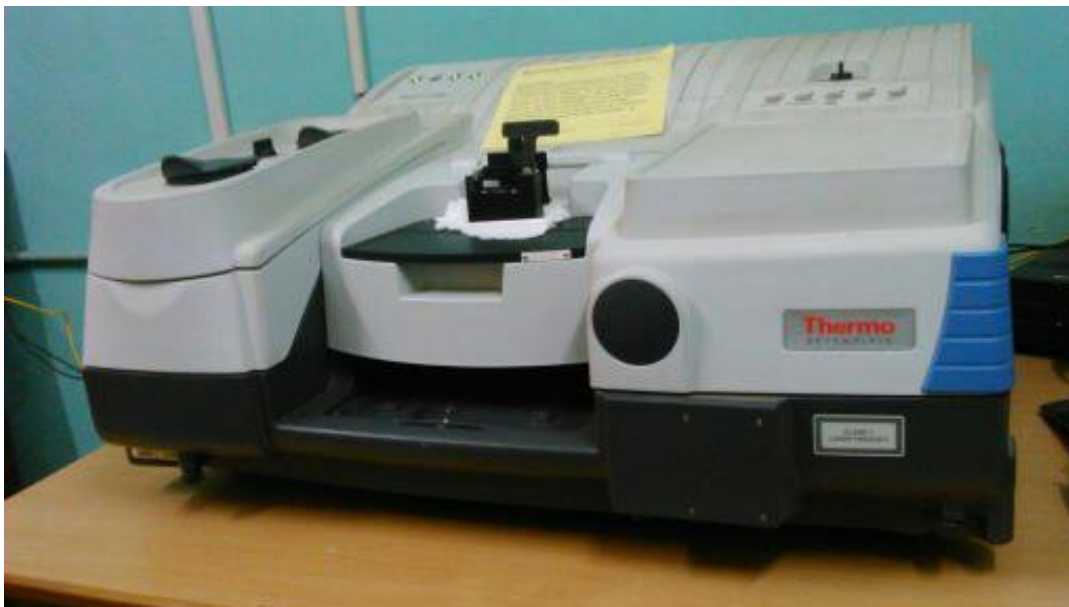
Figure 2.2 Thermo Scientific, Nicolet 6700, FTIR Spectrometer
