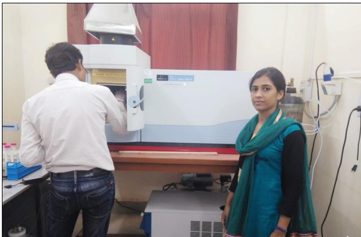
Fig. 3.11: Analysis of trace metals in water quality by ICP-ES instrument
