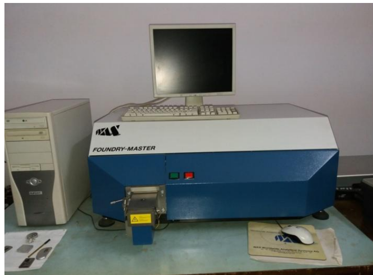
Fig.3.4 Optical Emission Spectrometer (Foundry Master)
