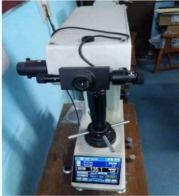
Fig.3.10. Vickers Hardness tester (Leco LM248 AT)
