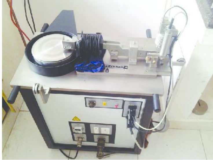
Fig.3.13. Pin-on-Disc type tribometer (DUCOM, TL-20, Bangalore, India)
