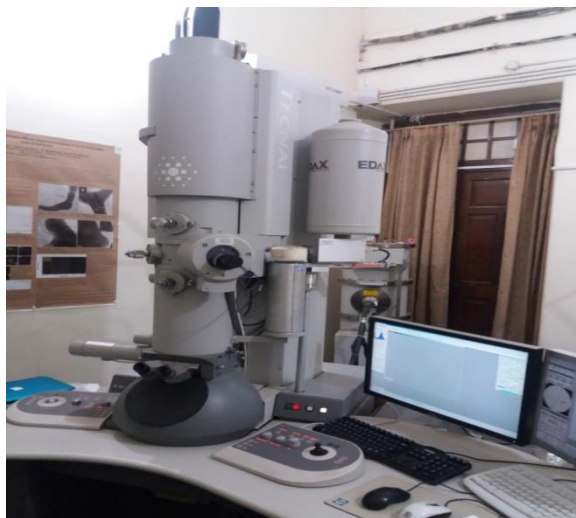
Fig.3.8. Transmission electron microscope (Tecnai G 2 -20)
