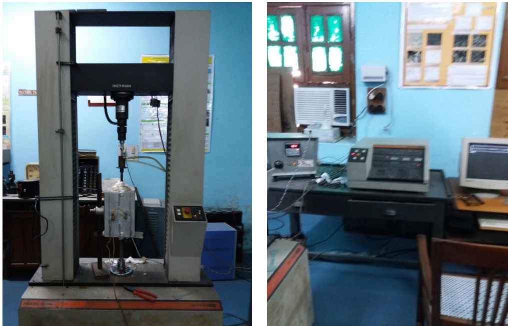
Fig.3.11. Instron-5848 tensile testing machine
