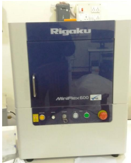
Fig.3.9. X-Ray diffractometer (Rigaku Miniflex 600 DTex)
