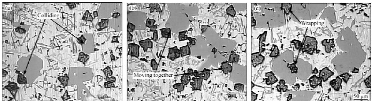
Fig.2.32. Mechanism of primary Si wrapping of Mg_2Si particles and adherence in the inner layer (Ref.97)
