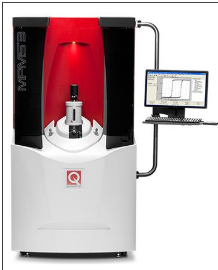
Figure 2.4 MPMS-3, Quantum Design (USA) used for magnetic measurement.
