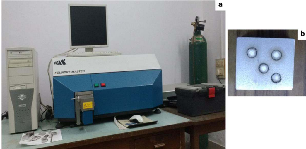
Figure 2.4 - (a) Optical emission spectrometer for chemical composition analysis of composites, and (b) composite sample after test.
