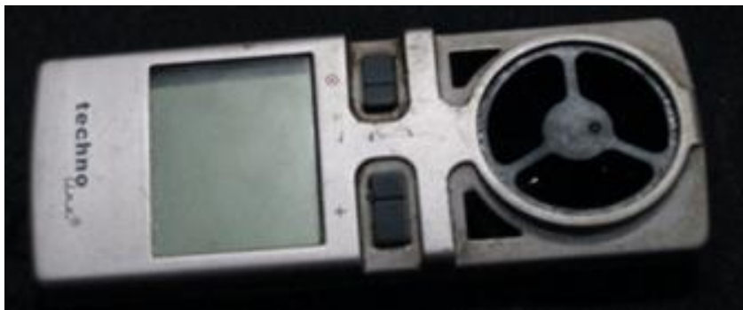
Figure 3.5: Photograph of anemometer to measure the velocity of gas flowing through pipe.
