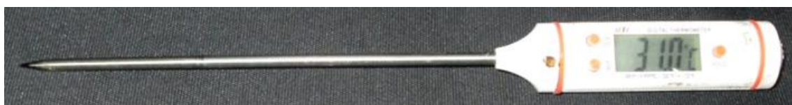
Figure 3.6: Photograph of digital temperature indicator to measure the temperature of gas flowing through pipe.
