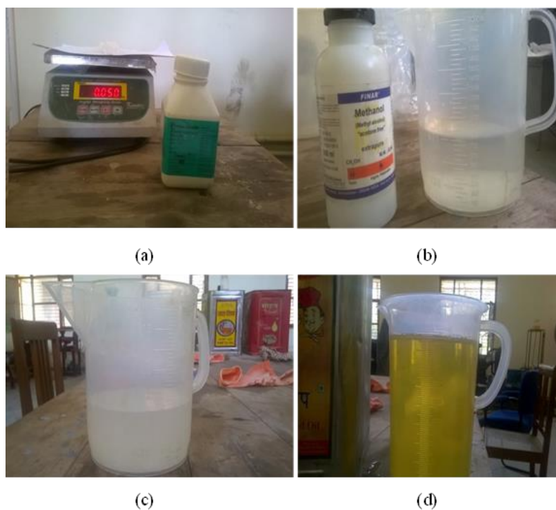
Figure 3.21: Soyabean methyl ester preparation, (a) Catalyst NaOH in 1% (w/v) of oil i.e. 50 grams. (b) Reactant methanol in 1:6 alcohol to oil ratio i.e. 833 ml. (c) Mixture of NaOH and methanol obtained by continuous stirring. (d) Soyabean oil.
