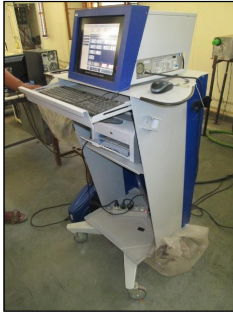
Figure 2.6: Gas chromatograph is used for measuring the different gas compounds present in the producer gas.
