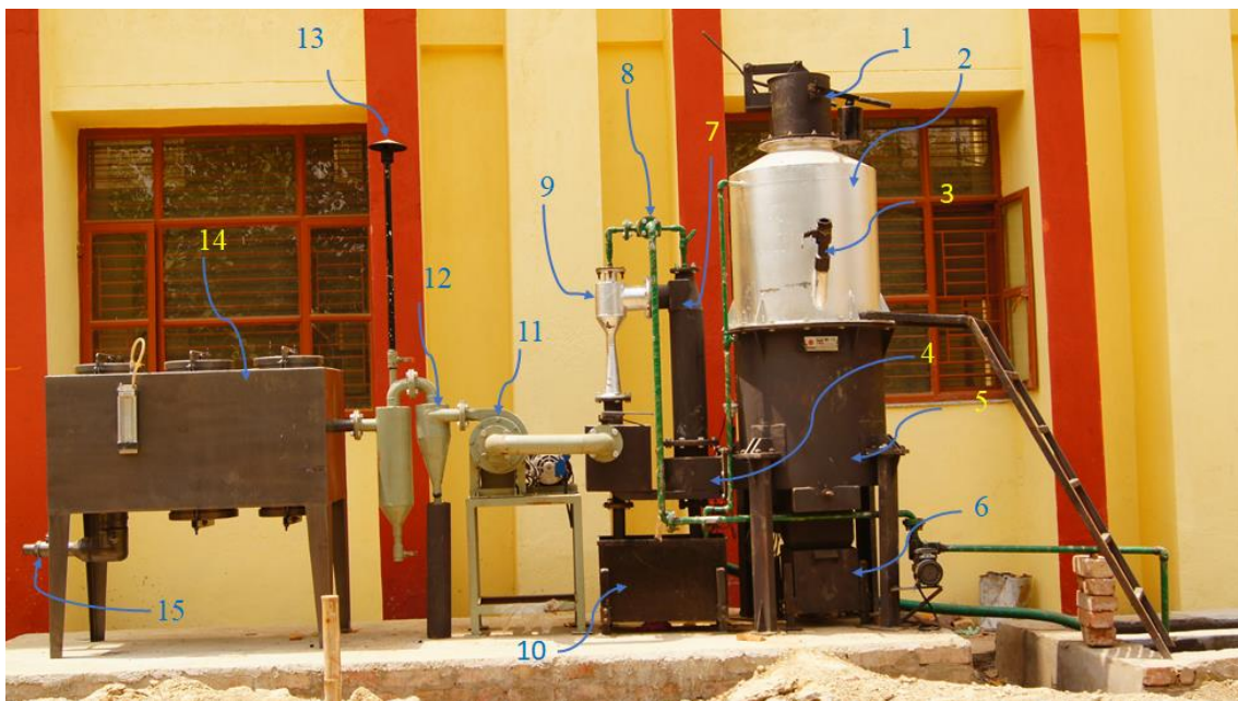
Figure 2.1: Downdraft gasifier system, an experimental setup for obtaining producer gas using solid biomass feedstock as a fuel. It is installed at IIT (BHU).
