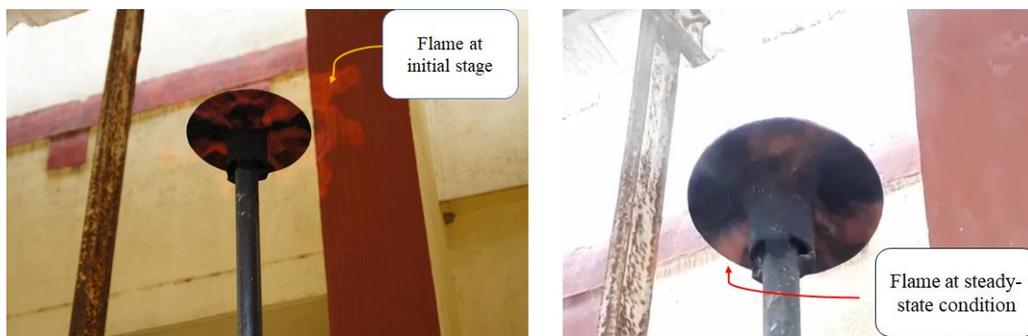
Figure 2.3: Quality gas test at chimney. The producer gas flame colour is an indication of its quality. At the beginning of the operation, the producer gas flame colour was misty red this is due to the presence of unburned gases, but later on, the flame colour turned uniformly dense red colour at the steady-state condition.
