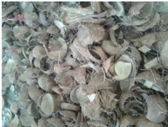
Figure 2.9: Coconut shell used as a solid biomass feedstock in downdraft gasifier system for obtained producer gas.
