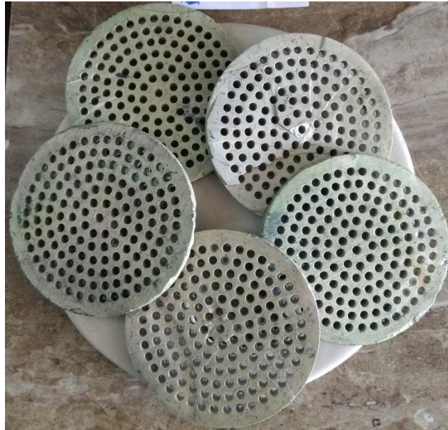
Figure 1.9: Shows the single layer catalyst coating in an alumina based circular hole perforated filters.
