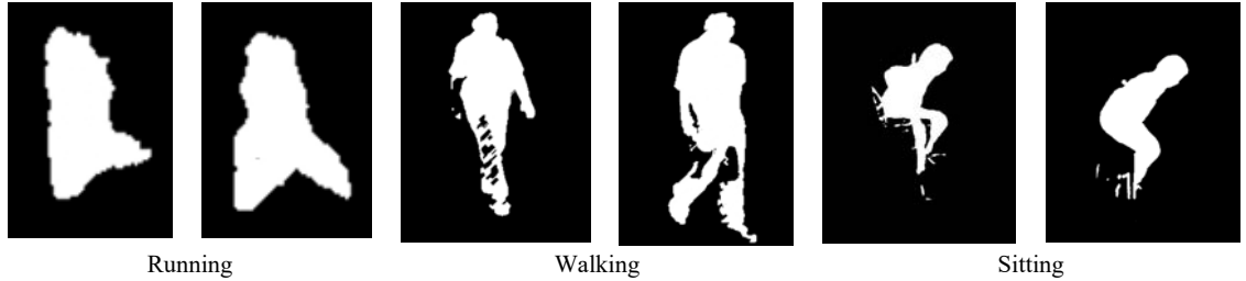
Figure 3.2: Threshold segmented image obtained after background subtraction for running, walking, and sitting activities of KTH, i3DPost and own dataset.
