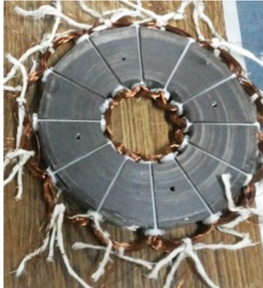
Fig. 1.12 Stator laminations of an Axial-flux permanent magnet generator.
