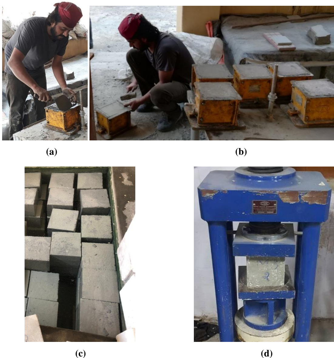
Figure 3.14 (a) Casting (b) Demoulding (c) Curing (d) Compressive strength test of 150 mm size concrete cubes
