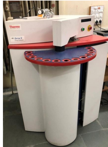
Figure 3.4 ARL OPTIM X X-Ray Analyzer for XRF analysis of OPC/RSA/MS
