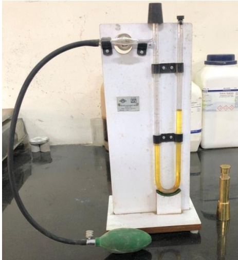
Figure 3.3 Blaine air permeability apparatus for specific surface area of OPC
