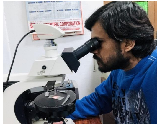
Figure 3.18 LEICA optical microscope for petrographic study of concrete specimens
