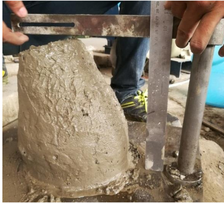
Figure 3.13 Slump test of concrete
