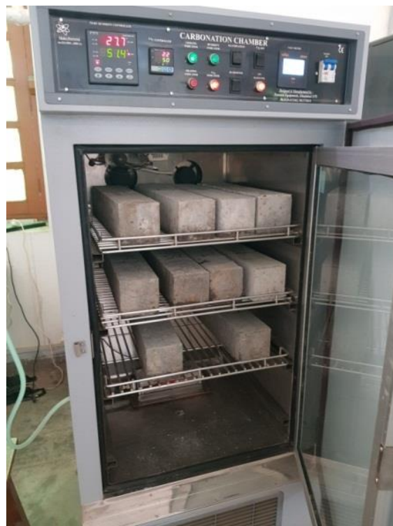
Figure 3.23 Concrete prisms in a carbonation chamber for ACC
