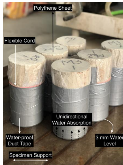
Figure 3.20 Setup for rate and coefficient of water absorption test of concrete
