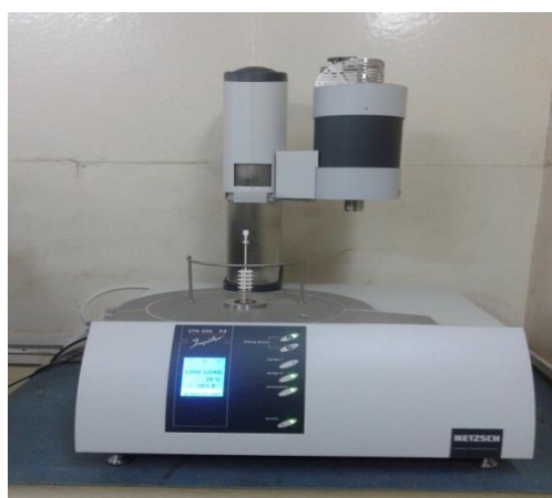
Figure 3.8 NETZSCH Thermo Gravimetric Analyser for TGA analysis of RSA
