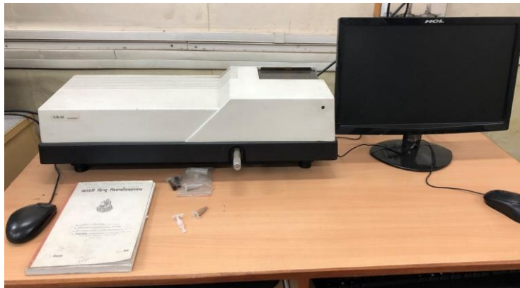
Figure 3.5 CIS-50 ANKERSMID particle size analyzer for particle size distribution of OPC, RSA and MS
