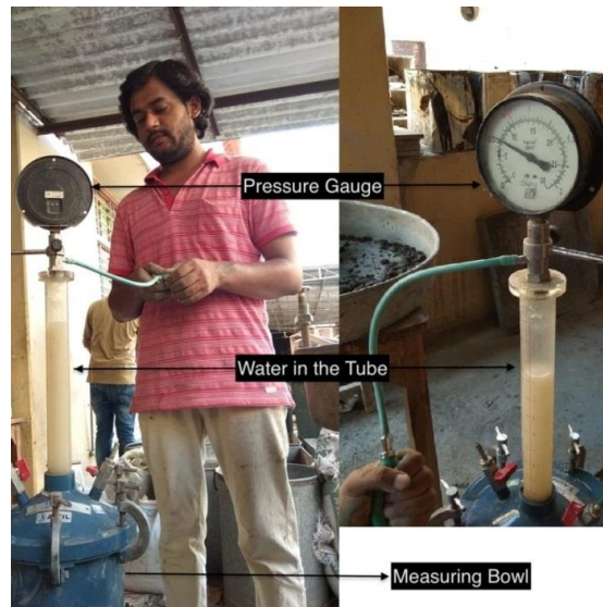
Figure 3.19 Set-up for air entrainment of fresh concrete
