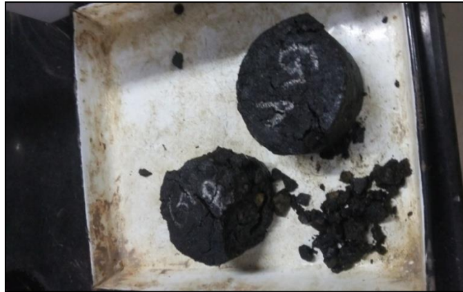
Plate 7.2 Untested GP 8.5% mix after being subjected to freeze-thaw conditioning
