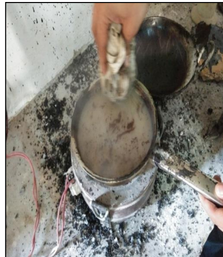
Plate 7.4 Skimming of free bitumen from top surface of boiled water
