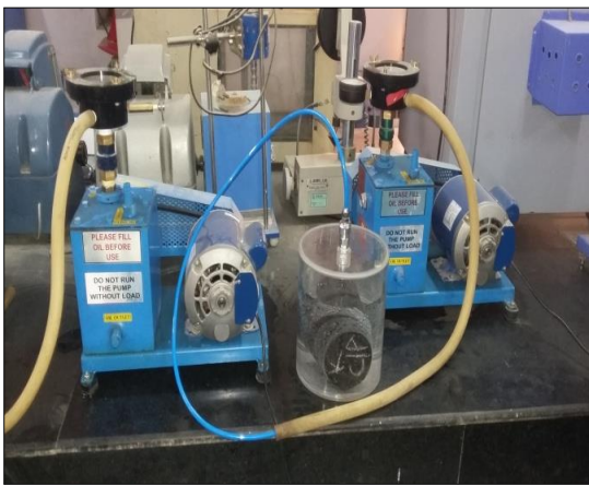
(a) Partial vacuum saturation of specimen
