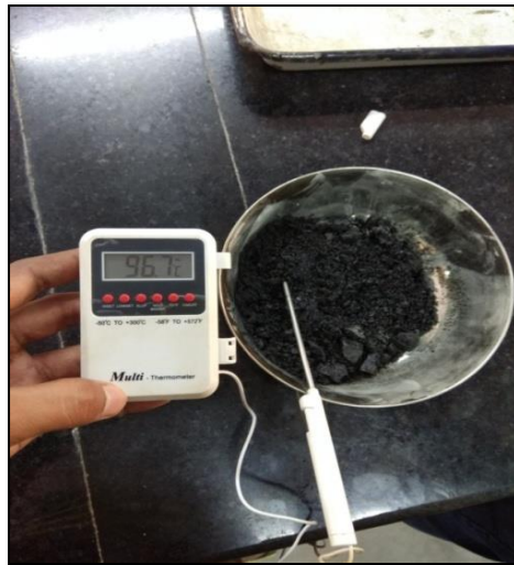
Plate 7.3 Measuring temperature of loose mix
