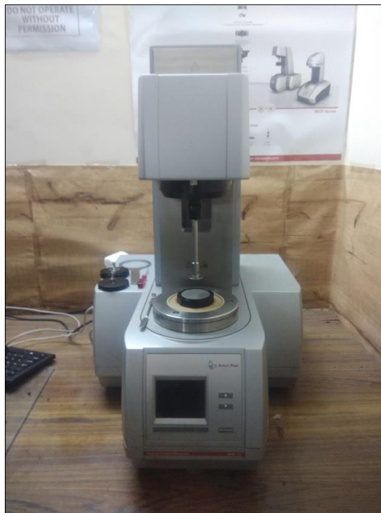
Plate 6.5 Dynamic shear rheometer used in this study (Anton Paar MCR 101)
