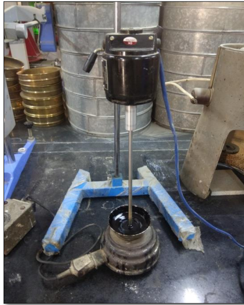
Plate 6.1 Preparation of bituminous mastic using mechanical mixer
