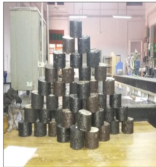
Plate 5.3 Marshall specimens after testing
