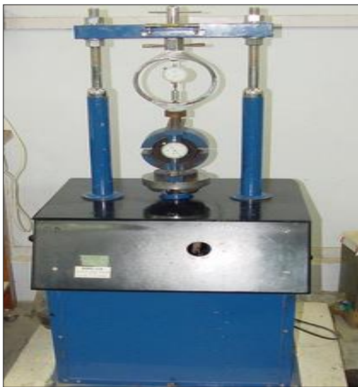
Plate 5.2 Testing of Marshall stability and flow
