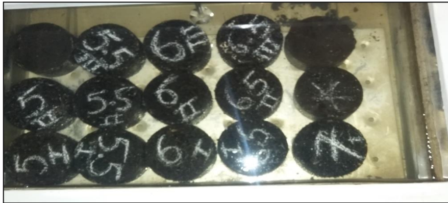
Plate 5.1 Conditioning of specimens in a water bath maintained at 60°C
