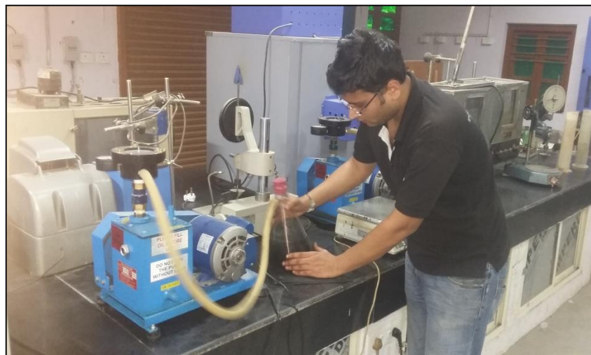
Plate 5.4 Determination of G_{mm} of mixes as per ASTM D2041 guidelines
