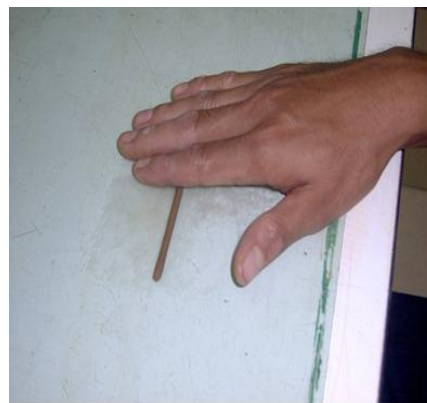
Plate 4.9 Determination of plastic limit
