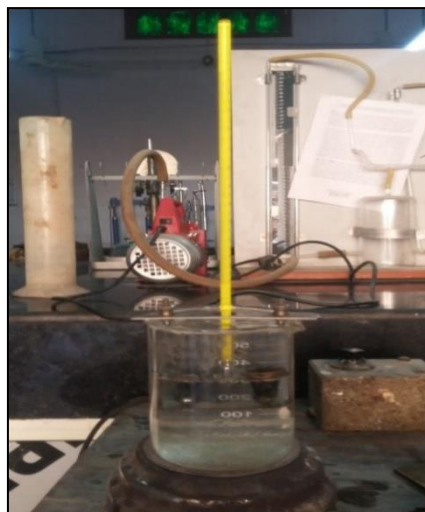
Plate 4.5 Softening point test of bitumen using Ring and Ball apparatus
