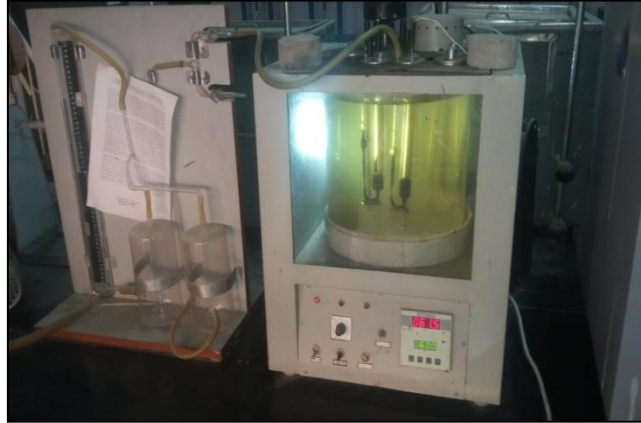
Plate 4.6 Determination of absolute viscosity using Cannon Manning viscometer in a viscometer bath
