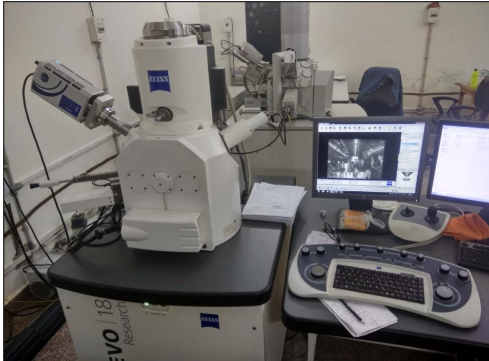
Plate 4.16 Set up for SEM at the central instrument facility, IIT (BHU) Varanasi
