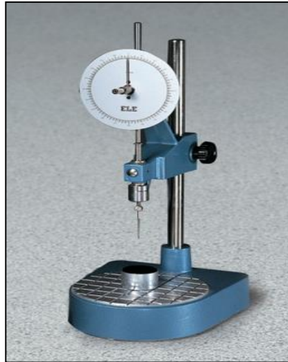
Plate 4.4 Penetration testing apparatus
