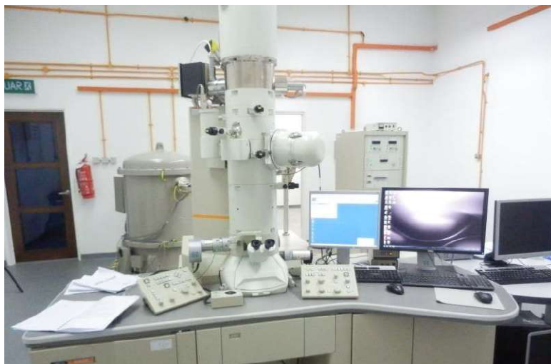
Figure 3.13 High-resolution transmission electron microscope measurement setup.
