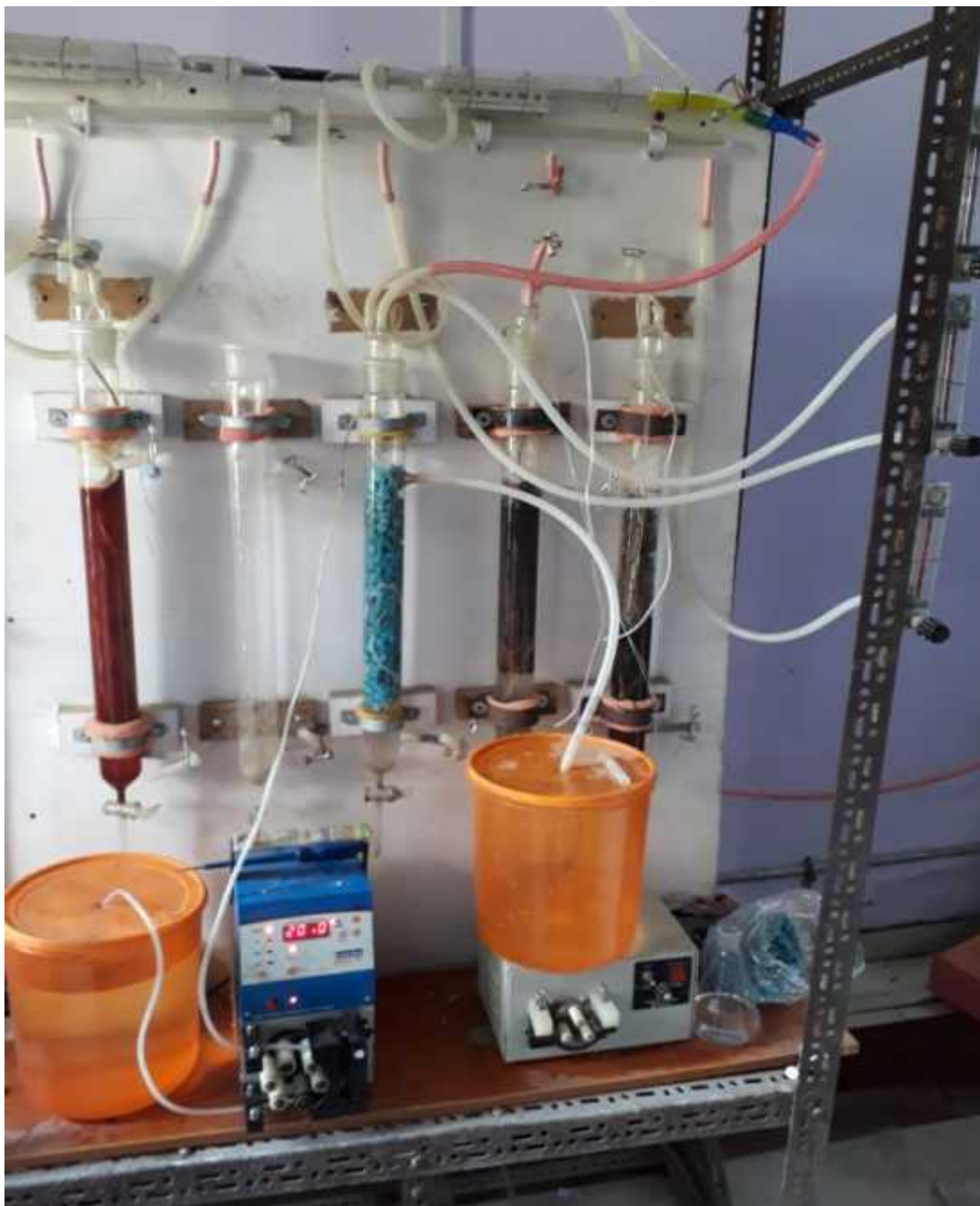
Fig.15 Image of experimental setup of continuous packed bed bioreactor
