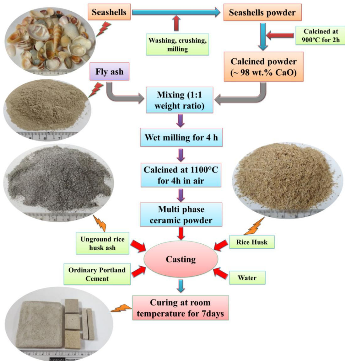
Figure 8.1 Preparation flowchart of ceramic board specimens.
