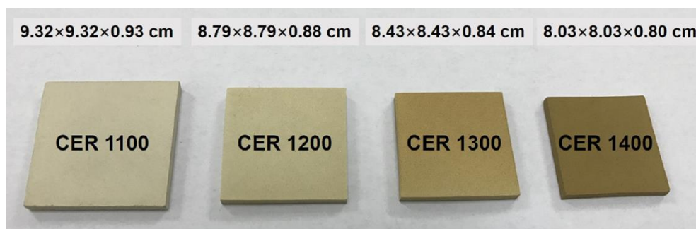
Figure 2.5: Photographs of fly ash containing mullite-based tiles sintered at different temperatures. Copyright with the permission from Ref. [ Luo et al. (2018b) ].
