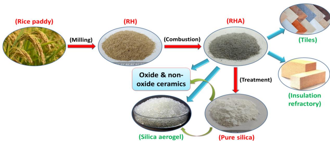
Figure 2.2: Schematic representation of the fabrication process of RHA and their application for the preparation of ceramics.
