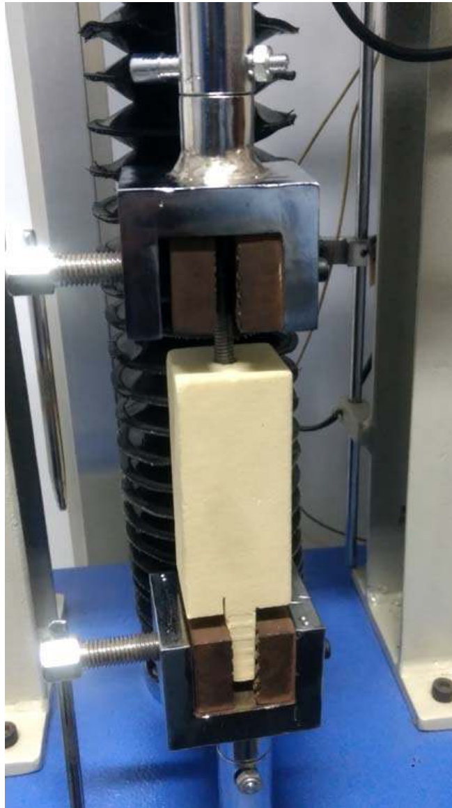
Figure 3.32: Experimental setup for measuring pull out strength of screw; setup shows the screw is inserted in the cellular rigid polyurethane foam block and fixed on the UTM.
