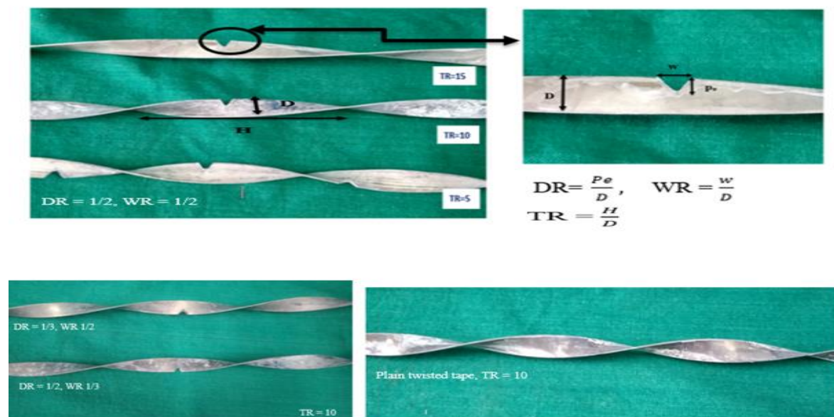
Figure 4.2. V-cuts twisted tape with different TR, DR and WR
