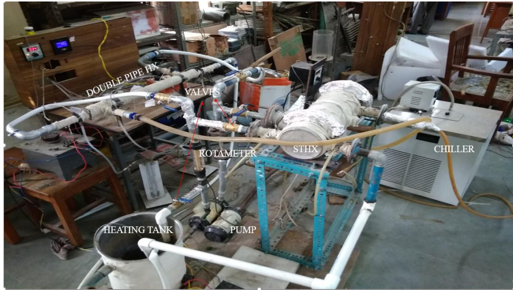
Figure 4.1 (b) Actual picture of the test setup
