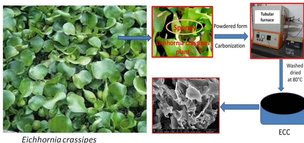
Figure 4.1 Schematic representation for the synthesis of ECCs.
