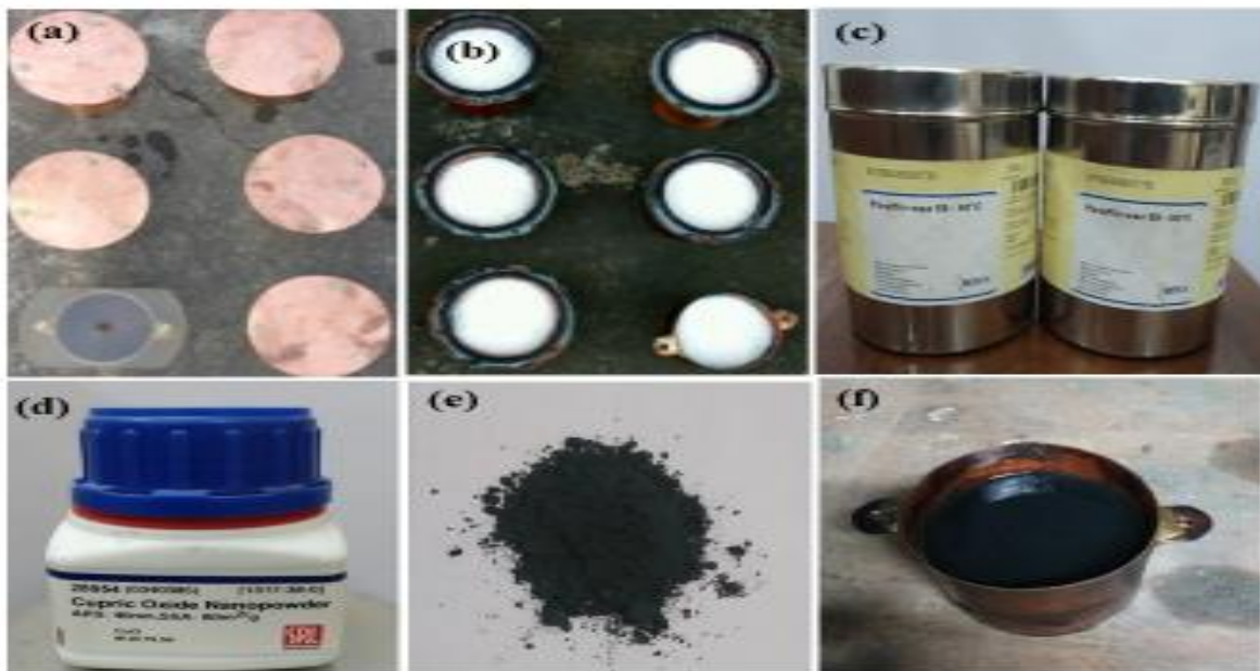
Fig. 4.3 A photographic view of (a) copper cylinders, (b) copper cylinders with PCM, (c) paraffin wax, (d) nanoparticle (CuO), and (e) copper cylinder with nanoparticle doped in
