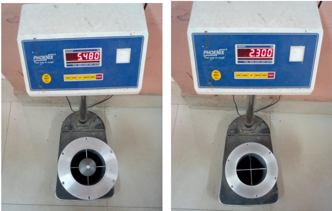
Figure 5.9. Weight of (a) SWG mode converter (reported in Chapter 3), (b) CSWG mode converter.
