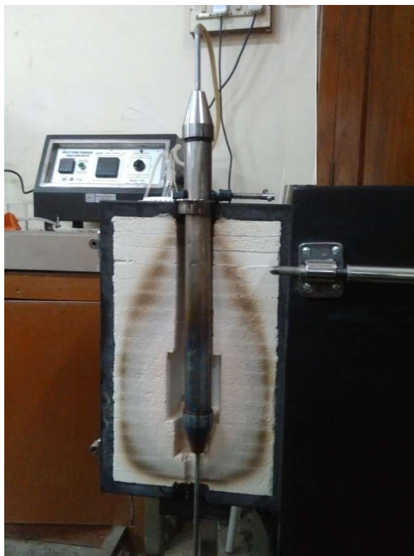
Figure 3.2 Single zone split tube furnace fitted with gasification column
