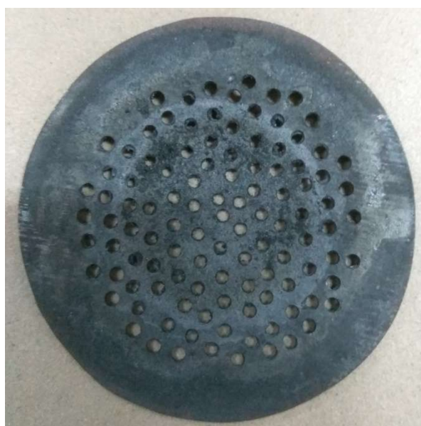
Figure 3.3 Inlet gas distributor cum support of bed inside gasification column
